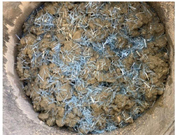
Figure 7: Concrete mix with 10 mm PET fiber.
