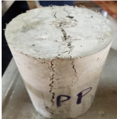
Figure 5: Sample of cylinder mix after testing.
